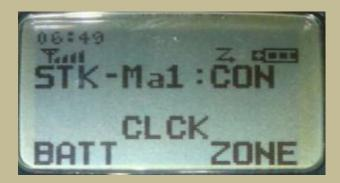
Turn the channel selector knob on the top of the radio clockwise one click to change to KMA2. To change back to the county dispatch channel, use the same steps as above but use the **Zone Down** button and turn the channel selector knob all the way counterclockwise. It does not matter whether you turn the channel selector knob or change zones first.
